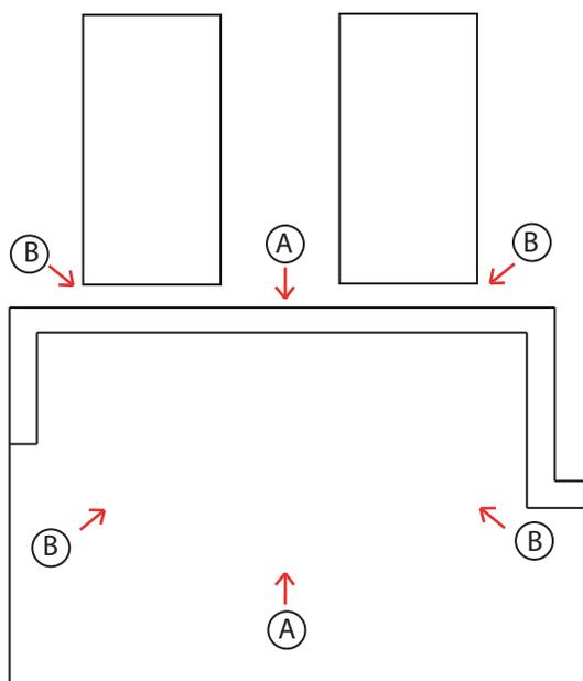
Red arrows indicate that water nozzles point to the center of the blast deck.
