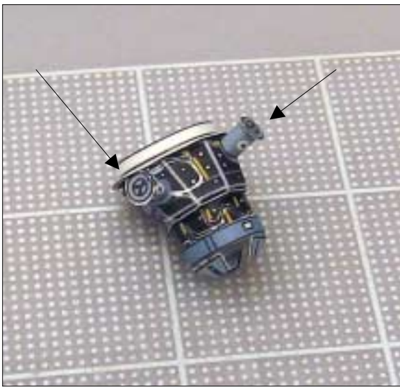
PMA-3 has two grapple fixtures as photo shows (arrows)
