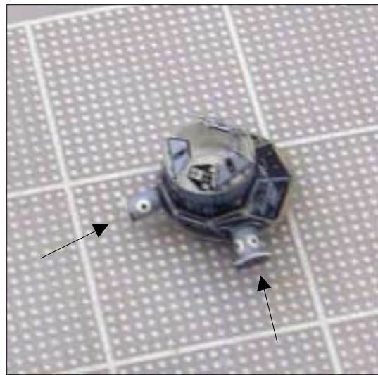
PMA-3 has two grapple fixtures as photo shows (arrows)
