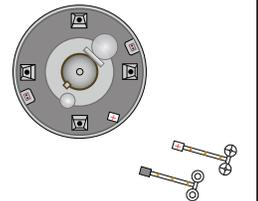
Docking Target to be placed on Zvezda Service Module (see manual)
