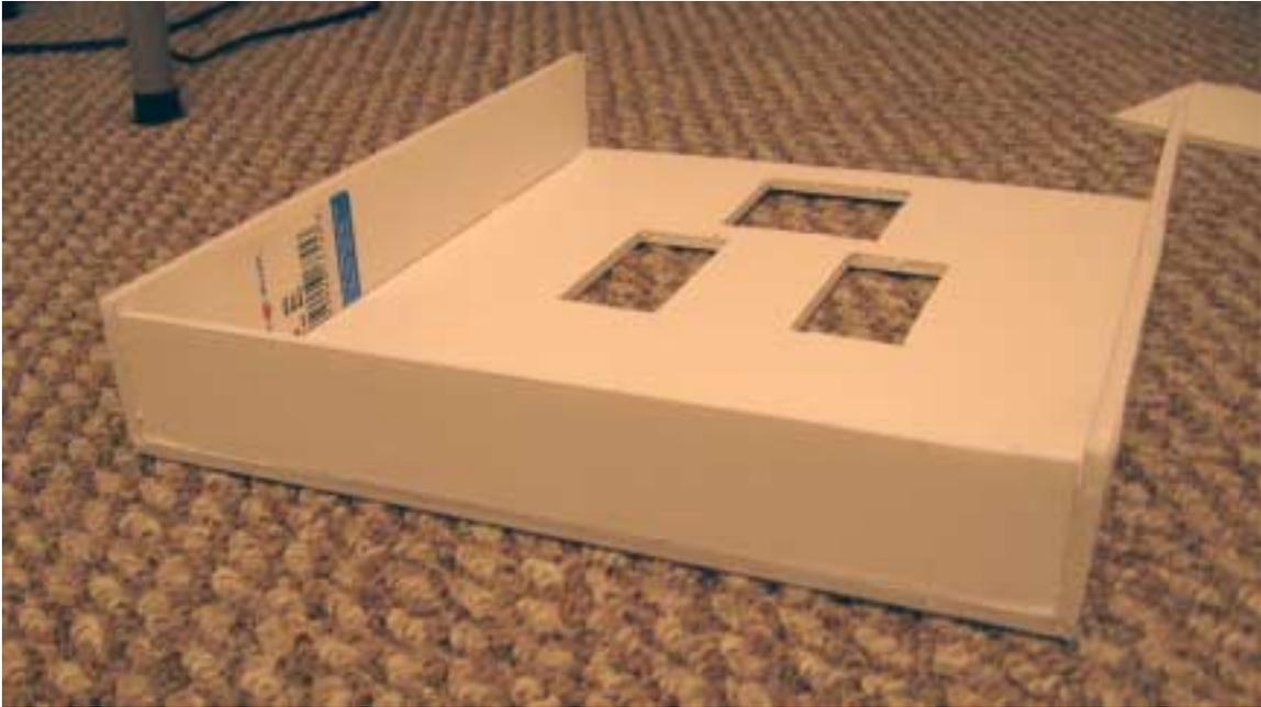
Next, glue the back part of the box. Notice that if cut with exact dimensions it will fit between the sides.
