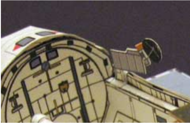
Note location of KU-band antenna that is glued on the tab from the right payload bay door.
