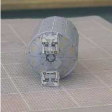
This photo shows the trunnion pin covers and the Grapple fixture in place for Space Station version module.
