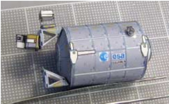
This photo shows the trunnion pin covers and the Grapple fixture in place for Space Station version module.
