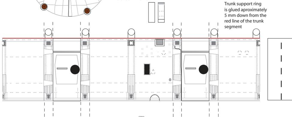
Trunk support ring is glued approximately 5 mm down from the red line of the trunk segment
