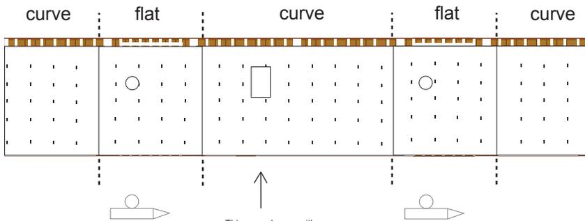
This curved area with the small rectangle is glued on the same side of the trunk that has the small rectangular box on the outside.
