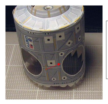
This photo belongs to the "Node hatches assembly manual" used for UNITY (STS-88) and HARMONY (STS-120) modules. First cut the 4 circular faces on the cylinder leaving the white circular area shown here (arrow).
