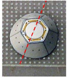
The red arrow indicates where the seam is. The hexagonal shape part is glued underneath.
