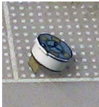
The Power and Data Grapple Fixture is glued on the keel side in an angle.
