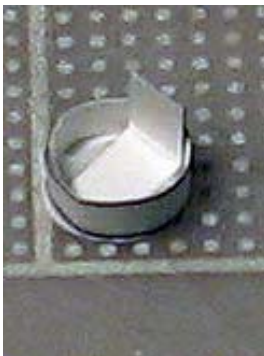
The Power and Data Grapple Fixture is glued on the keel side in an angle.
