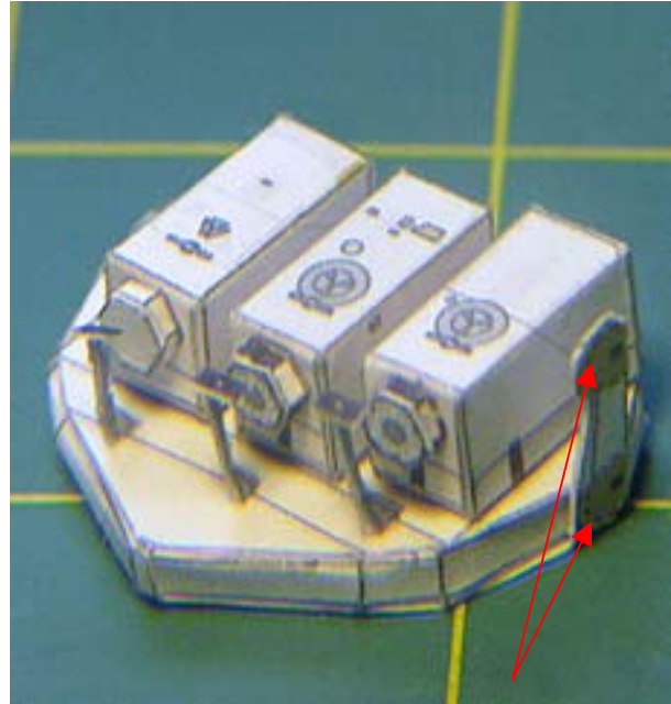
Note location of the visual targets for each of the EF payloads and the trunnions (red arrows).
