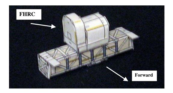
Note the position of the Flex Hose Rotary Coupler (FHRC) on top of the LMC.
