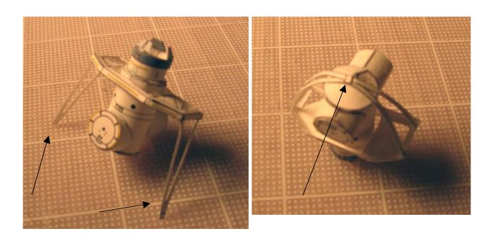
Photos show the position of the other elements when building this Docking System. Note how the side thin parts are glued at the bottom of the Docking System.
