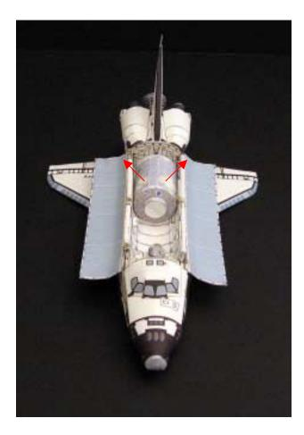
This photo shows how the Node 2 module is placed on the payload bay. Notice the ports in an angle and the logos for orientation.
