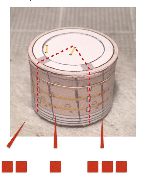
Follow the guidelines from this photo. The gray areas need to match the small white rectangles on the body of BEAM and in between it has to be the single orange square section.
